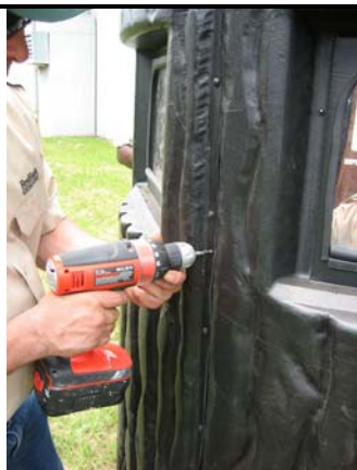
18. Drill from inside and screw from outside with #8-32 x 3/4" SEM screw.
