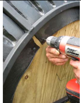
26. Fasten bottom blind lip to plywood floor with (3) #8 -32 x 3/4" SEM screws in each panel.
