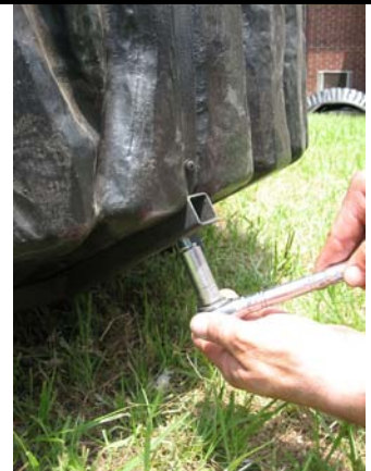
29. Fasten bracket to blind with 2" x 5/16" bolt inserted from the outside and 5/16" flat washer, 5/16" lock washer and 5/16" nut on inside. Repeat on other two support brackets. Install (3) 1" plastic caps in ends of support brackets.
