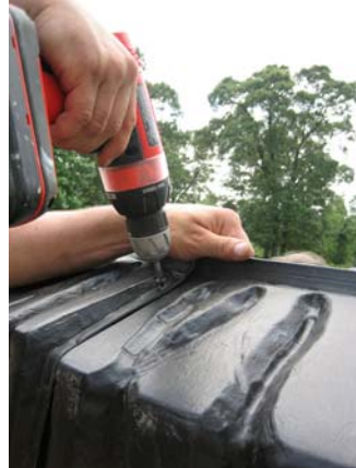
10. Fasten with #8-32 x 3/4" SEM screw and speed nut.
