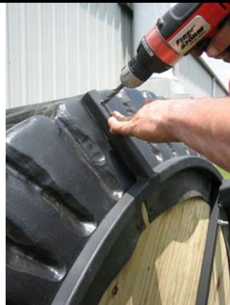
28. While blind is still on its side using hole in ring support bracket as a guide, drill a 5/16" hole through bottom seam.
