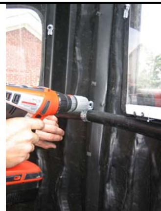
17. Install single clamp between the remaining windows keeping pipe aligned with the bottom of the windows.
