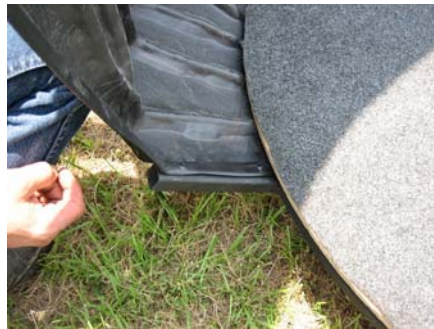
4. With door centered with the ladder brackets side lip of side panel should line up with tower ring support bracket.
