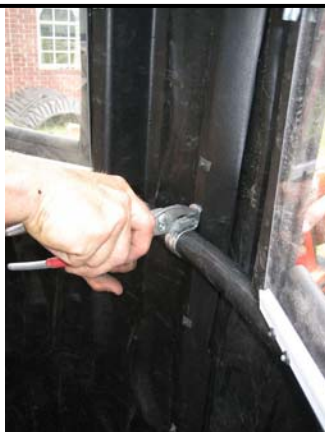
19. Use speed nut on inside over clamp.
