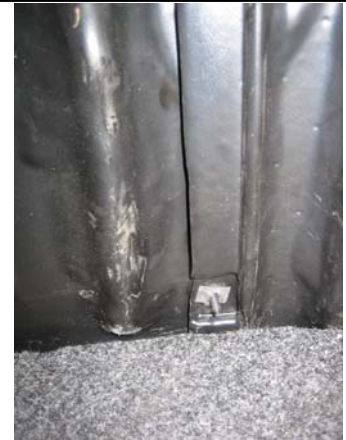
8. After screw penetrates both panels place speed nut over screw and keep turning until nut pulls tight (use pliers to hold speed nut).
