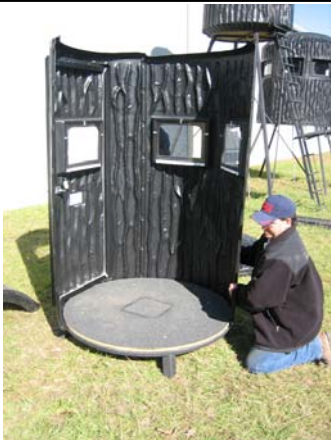
6. Insert second panel the same as first.
