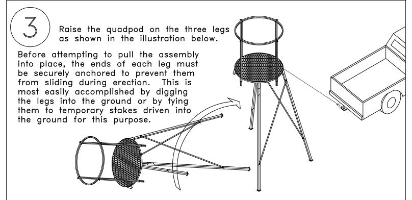
CAUTION: Never stand under or near the QuadPod as it is raised to its full upright position. Use extreme caution to prevent pulling QuadPod past vertical.
